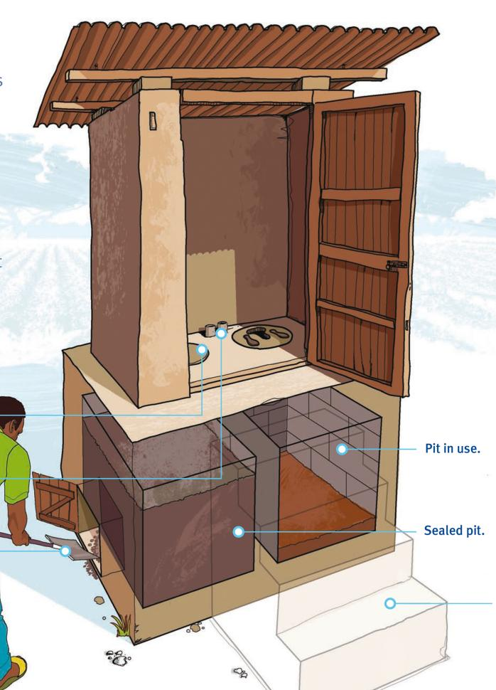
The structure can be raised in areas with a high water table or where the ground is very hard.
